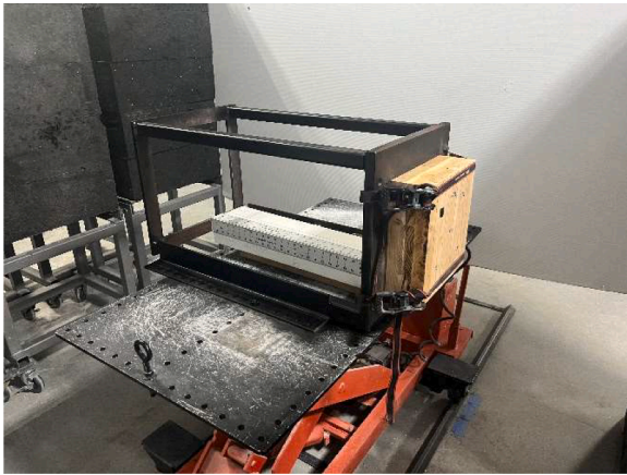
Fig. 3. CLT target specimen and fixture.
