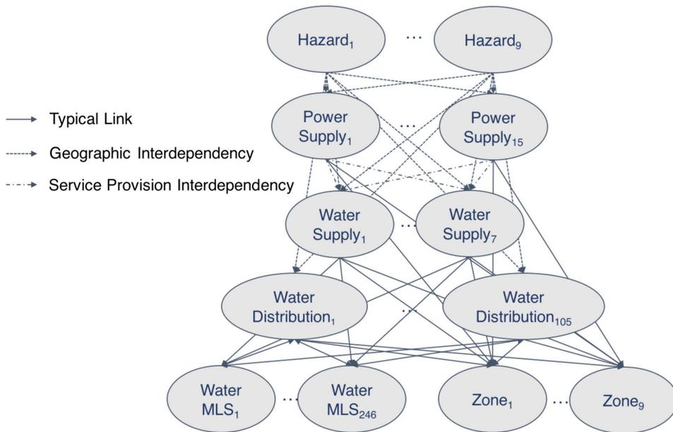
**Fig. 8.** Overall BN model of Atlanta water and power distribution networks.
