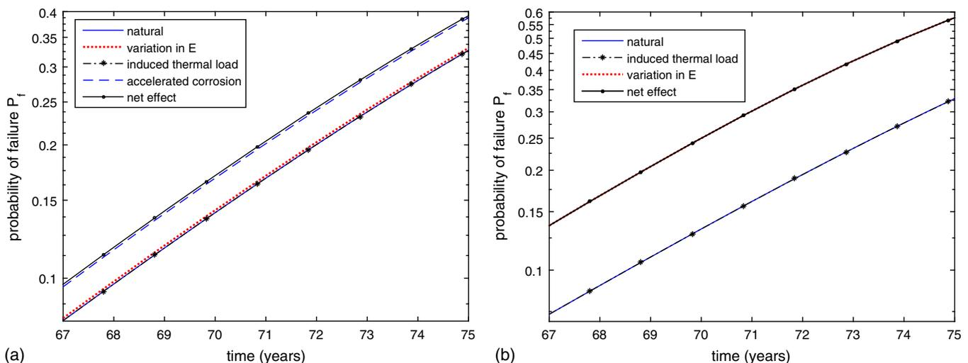
**Fig. 2.** Probability of failure of example: (a) steel; (b) wood structures with change in resistance caused by environmental factors
