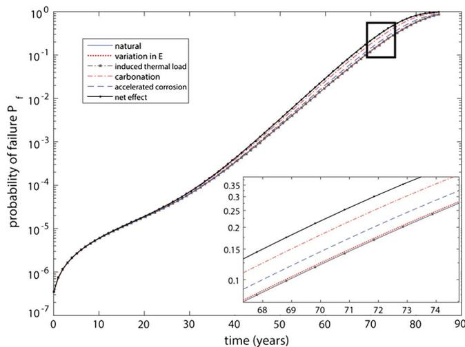
**Fig. 1.** Probability of failure versus time, with changes in resistance caused by environmental factors
