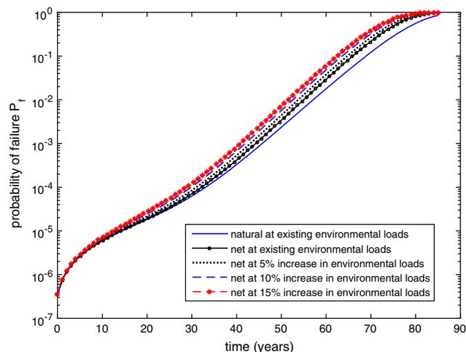
**Fig. 3.** Probability of failure versus time, with increase in the extremes of loads, corresponding to an increase of 5, 10, and 15% increase in the mean in 100 years
