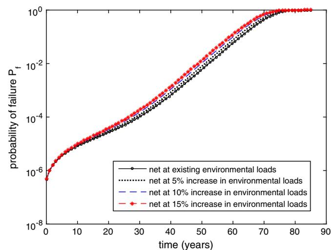
**Fig. 4.** Probability of failure versus time, in which two different significant load events act on the structure
